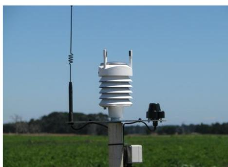
Figure 9. The Vaisala WXT520 weather station.
