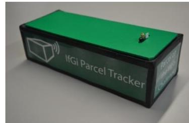
**Figure 1 - The sensing device that can accompany a parcel to track and monitor its parameters.**
