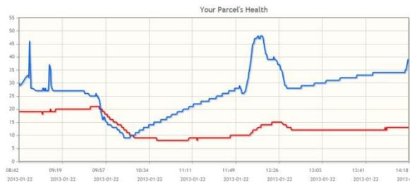
**Figure 3 - The temperature (red) and humidity (blue) measured within a parcel on the test ride.**
