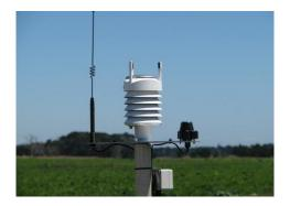
Figure 9. The Vaisala WXT520 weather station.
