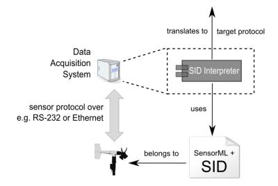
Figure 4. Translation of sensor protocol by an SID interpreter.
