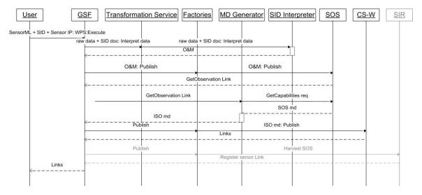
Figure 6. Sequence diagram for sensor data publication and registration into GIIs.
