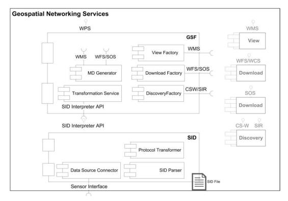
Figure 5. Detail of the Service Model for sensor data interpretation and publication in GII (in UML notation).
